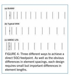
dipole; the width of the loop is significantly greater. Like the closely spaced parasitic director, the loop feed requires some space along the boom, and that in turn requires a significant reorganisation of all the other element lengths and spacings. However, the different method of excitation creates its own characteristic effects on the performance of the Yagi and by careful optimisation GOKSC has created a new range of direct feed Yagis that have excellent gain, pattern and bandwidths.
